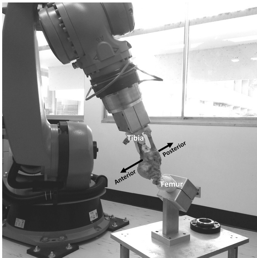
Fig. 4 Robot for mechanical testing of anterior tibial laxity.
